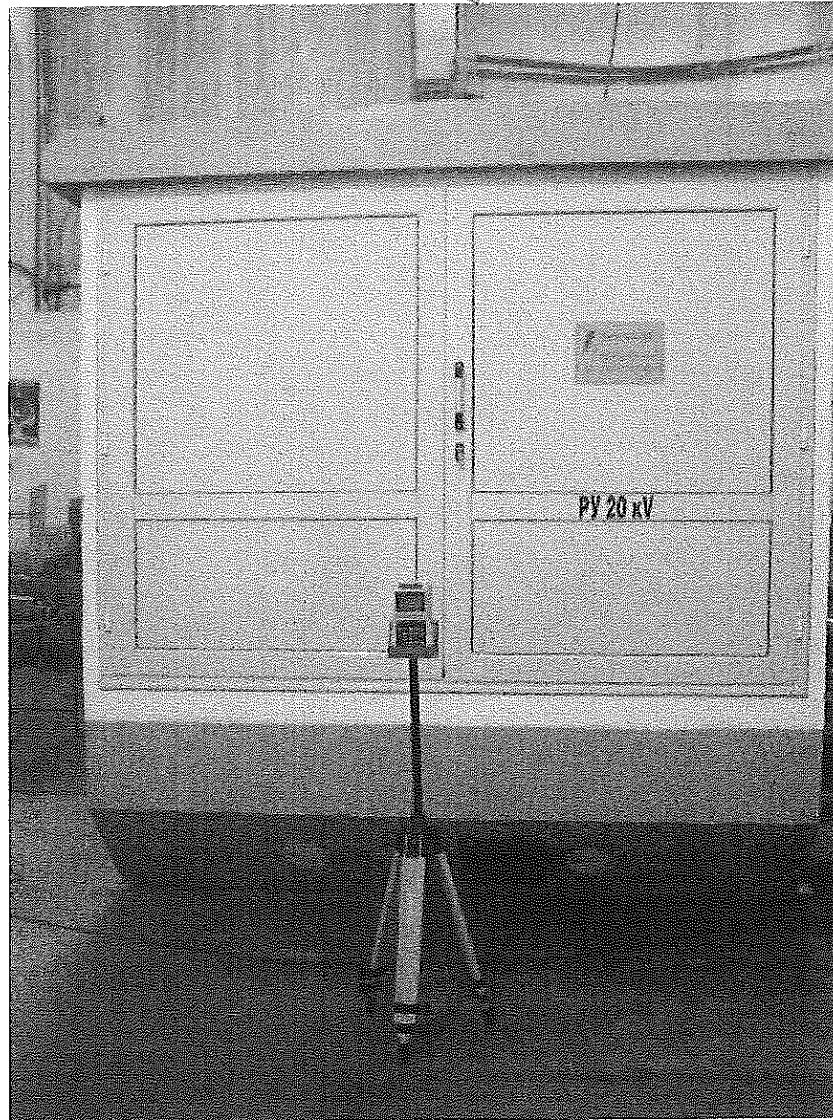
Test set-up for measurement of magnetic field
